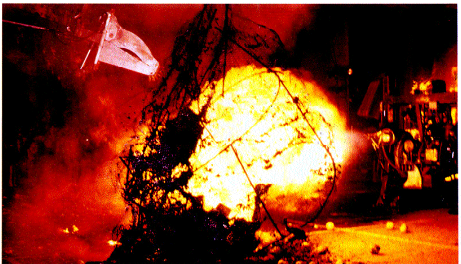
Alpha's XTRA•GUARD 5 cable installation in the robots "Big Arm" has survived the torture of a half-dozen performances and dozens of rehearsals. The cable's FEP-Teflon jacket is rated to +200°C without wiring burn-through.
